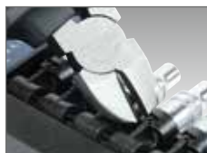
Unlocking the holder through removing the protruding hook.
